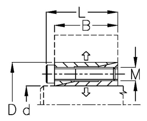
B mm = 13d mm = 12.00D mm = 22Fit tolerance = Aksel h8, Nav H8 F kN torque = 3.0L mm = 15.5M mm = M2,5P N/mm2 surface pressure on shaft/hub = 50 Surface roughness = R? ?  $3.2 \mu n$ T N m torque = 20Ts N m bolt tightening torque = 1.2
